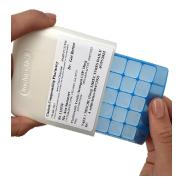
STEP 3: Slide protective cover over tray to activate the CLICK locking mechanism.
